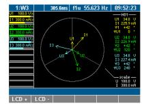
Vector display of HO1 up to 6 signals. For easy testing of the right connection of the instrument and quick overview of the phase angle of each signal.
